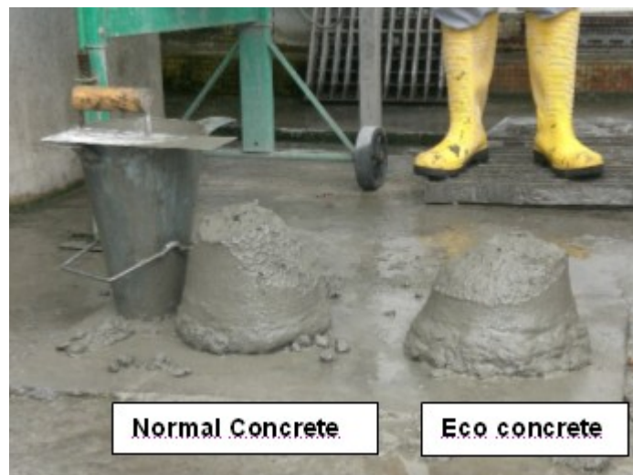
Figure 25: Slump test comparison for normal concrete versus eco concrete
